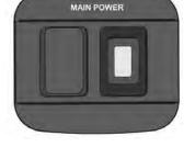
during periods of storage or during maintenance. The solenoid must be engaged for the 12-volt house electrical system to operate. Never depress the momentary battery disconnect switch for longer than 1 second. Depressing and holding the switch down will disable the battery disconnect solenoid. Should this occur the main ground cable for the house batteries must be removed for 1 minute to re-enable the solenoid operation.
