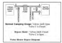
3-valve water heater bypass
