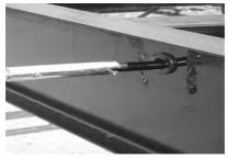
Fig. 1 Through Frame Cranck Extension w/pin
